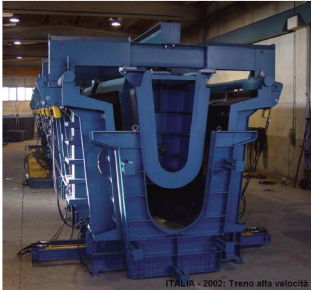
“U” SHAPE BEAM SELF REACTING MOULD
