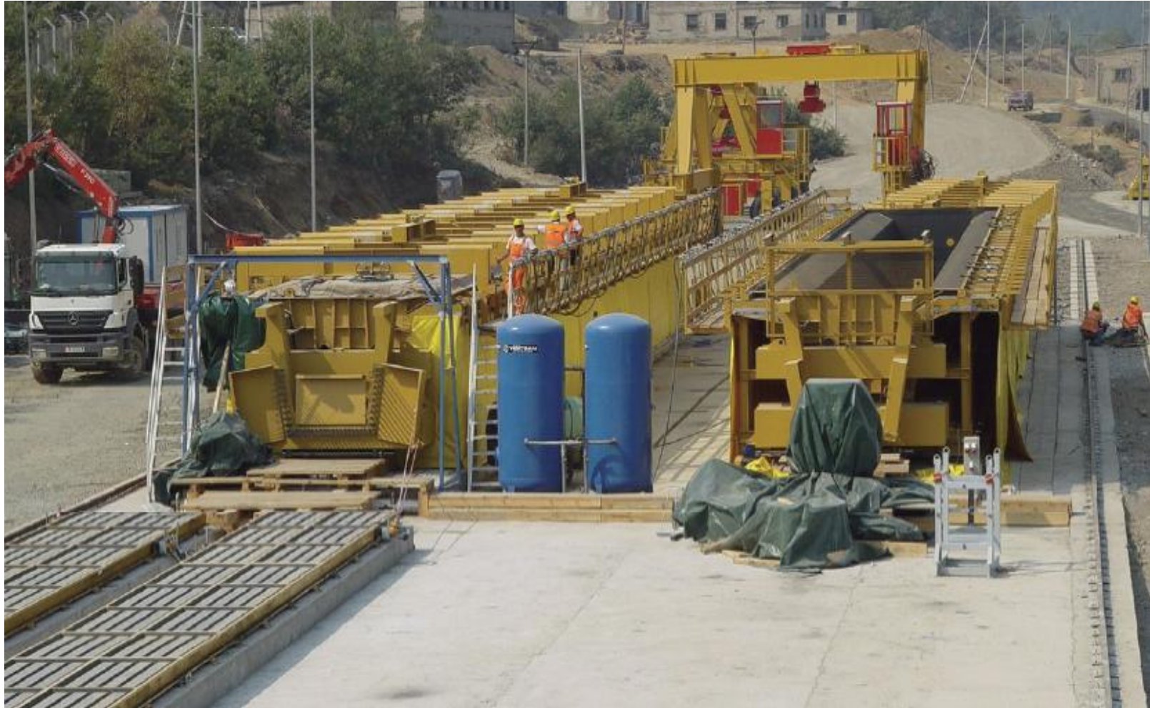
“U” SHAPE BEAM SELF REACTING MOULD
