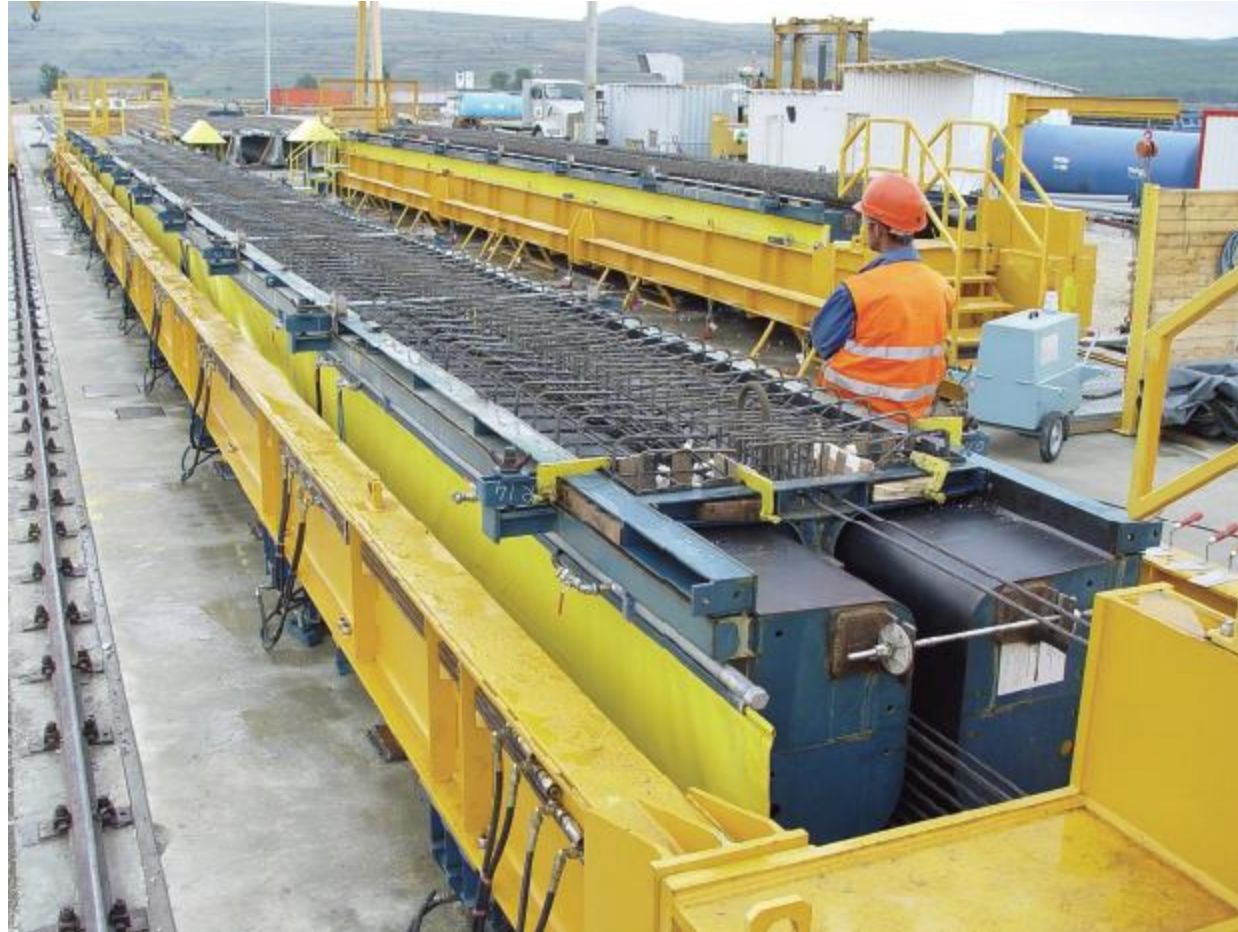
“T” SHAPE BEAM SELF REACTING MOULD
