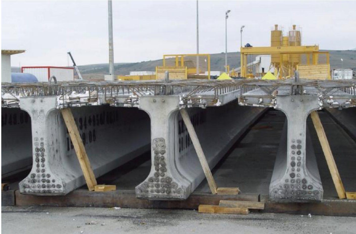
T” SHAPE BEAM SELF REACTING MOULD
