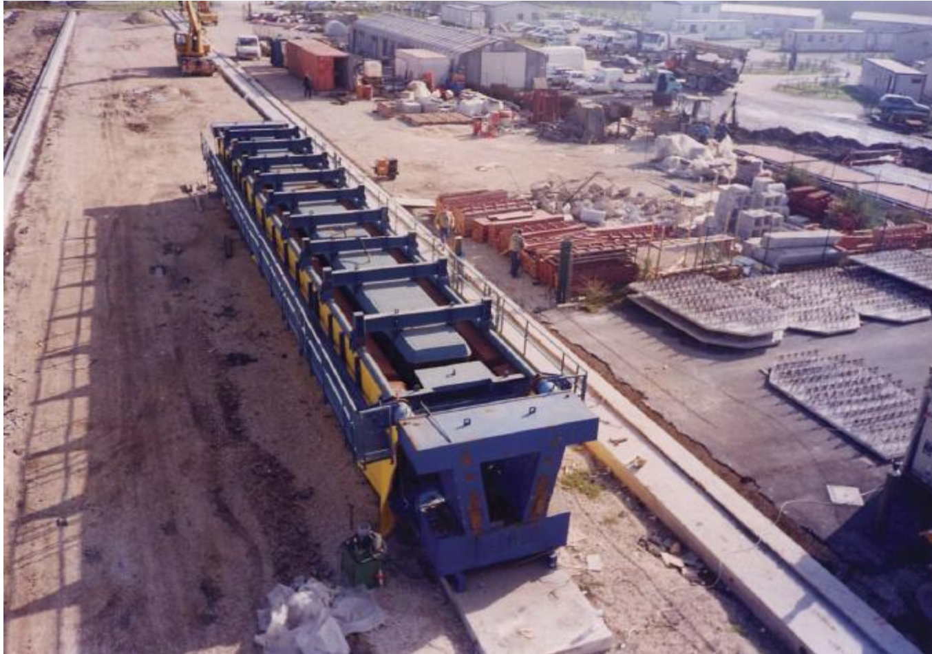
“U” SHAPE BEAM SELF REACTING MOULD
