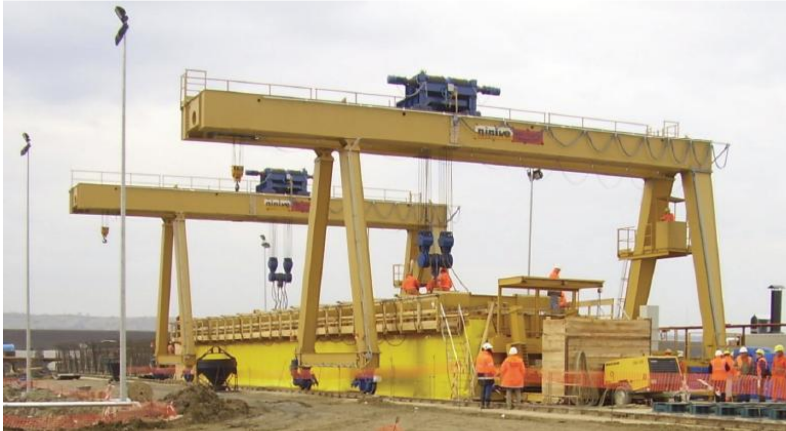
“U” SHAPE BEAM SELF REACTING MOULD
