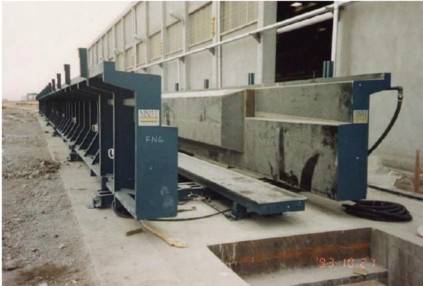
T" SHAPE BEAM CONVENTIONAL MOULD & DRAWING BACK FLANKS
